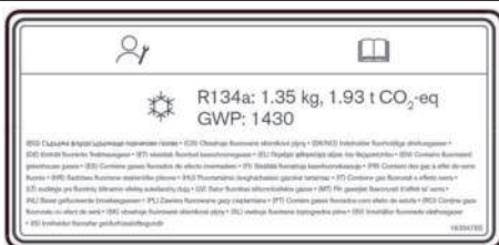
26. The air conditioning system is filled with R134a. Spare part number: 16354765
