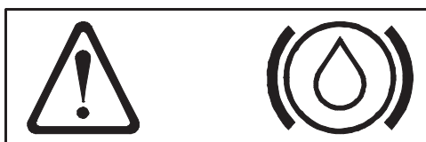
Brake cooling oil level low
