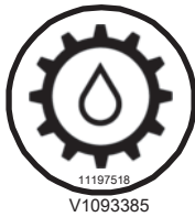
5. Oil fill point transmission Spare part number: 11197518
