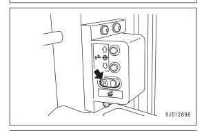
3. Hold down the power ON/OFF and menu switch to turn on the control box power.
