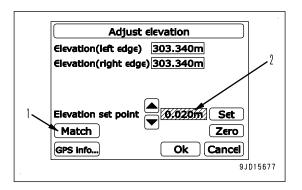
5. On "Adjust elevation" screen, press "Ok" (3).
