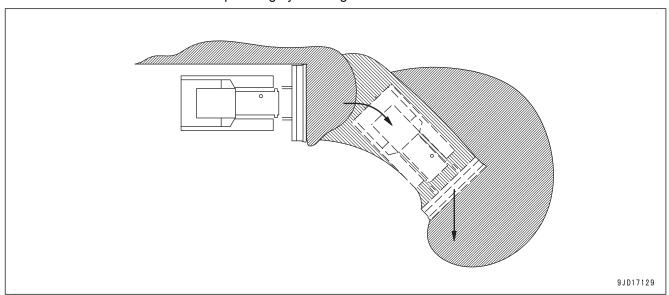
If you face the blade straight forward by angling operation, less soil spills from the sides of the blade.
