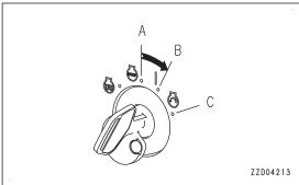
Check that LED of the back grade mode switch lights up for 3 seconds when turning the starting switch to ON position.
