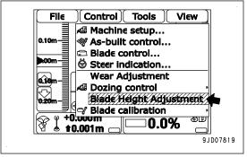
3. On "Blade Height Adjustment" screen, check the blade elevation adjustment value before adjustment, and calculate compensation value (a) to input.
