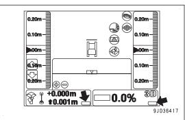
"Auto Control Disengaged!" message pops up on the control box screen when the blade automatic control is switched from on to off.
