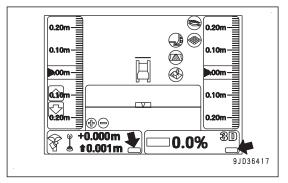
While the back grade mode is turned on, you can perform leveling work even in reverse travel since the blade automatic control also operates in reverse travel similarly to in forward travel.
