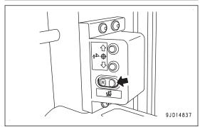
LED of the back grade mode switch lights up, and the back grade mode indicator is displayed at the top of "AUTO" on the control box screen.
