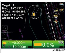
When the point to navigate to and the machine are displayed on the same screen, the arrow goes out.
