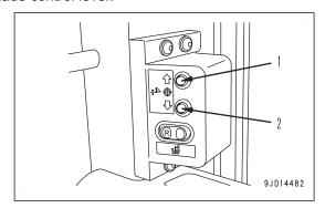
The increase/decrease amount when the cut/fill offsets switches are pressed is the same as the setting of the "Cut/Fill offsets" on the control box screen.
