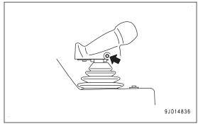
The blade automatic control is turned off also when operating the work equipment lock lever by holding the operating portion on the top and placing the lock lever in LOCK position (L).
