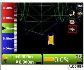
"Auto-Topo:" (information set on detailed position screen) and topographic survey recording are displayed.
