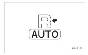
While the back grade mode indicator is displayed on the control box screen, you can control the dozing in forward travel by setting the joystick (steering, directional and gear shift lever) to FORWARD position (F). You can perform the back grade work by setting the lever to REVERSE position (R).
