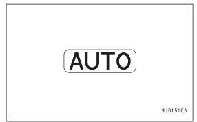
While the back grade mode is turned on, if the blade automatic control is turned off ("AUTO" on control box screen goes out), the back grade mode is automatically turned off.
