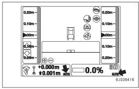
When the back grade mode is turned on, LED of the back grade mode switch lights up, and the back grade mode indicator is displayed at the top of "AUTO" on the control box screen.
