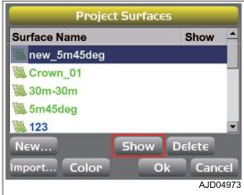
A check mark is inputted to "Show", and the content of Surface is displayed on the main window.
