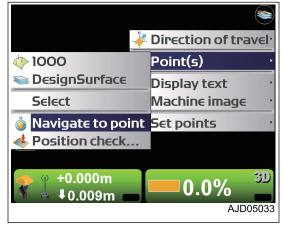
The result of navigation to the point is displayed on the main window.
