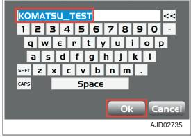
10. Check that the information of the point is input to "Point description:", and press "Ok".
