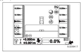
When turning on the back grade mode again, press Auto/ Manual switch (1), turn on the blade automatic control, and press back grade mode switch (2).
