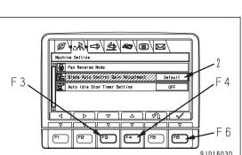
Select "Default" (4) on "Blade Auto Control Gain Adjustment" screen and press switch F6.
