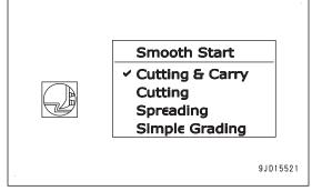
Use the automatic control of blade to cut and finish the curved surface which does not have an inflection point.
