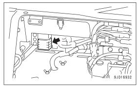
1. Hold down the power ON/OFF and menu switch to turn off the control box power.
