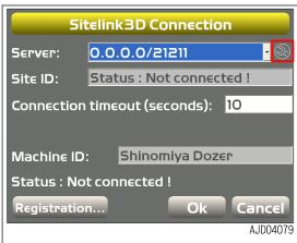
4. Input the address of the server and the site No. which have been checked in the WebPortal, and press "Ok".
