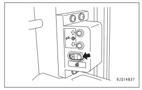
When the back grade mode is turned off, LED of the back grade mode switch goes out, and the back grade mode indicator on the control box screen goes out as well.
