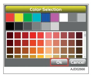
5. On "Section" tab, press "Color", and change "Section/ profile line color: " or "Show grade transitions:".
