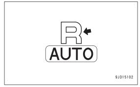
While the back grade mode is turned on, when the joystick (steering, directional and gear shift lever) is set to reverse position (R), the blade automatic control operates as well similarly to when the lever is set to FORWARD position (F).
