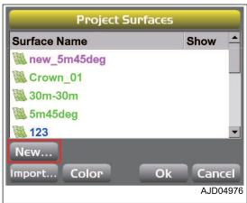
4. On "Surface Name and Type" screen, press the input section for "Name".
