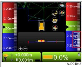
However, when adjusting the lateral slope angle of Surface, you are required to use the slope fixing function.
