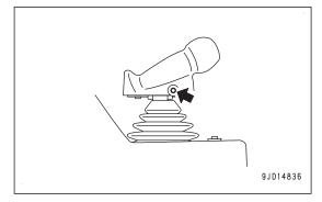
When the blade automatic control is automatically turned off, "Auto Control Disengaged!" message pops up on the control box screen, and notice sound "Beep" can be heard.
