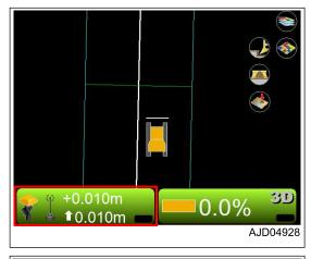
"Adjust elevation" screen is displayed. ("Set" is displayed in red.)
