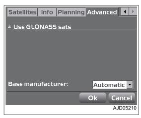
When both of the machine and the base station use GLONASS and the base station is not manufactured by Topcon, select an applied base station manufacturer such as Sokkia, Trimble, etc. from "Base manufacturer:" list.
