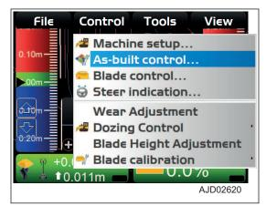
3. On "As-built Control" screen, select the As-built Surface to be deleted, then press "Trash" button.
