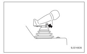
The blade automatic control is turned off also when operating the work equipment lock lever by holding the operating portion on the top and placing the lock lever in LOCK position (L).
