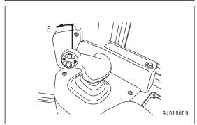
4. Hold down the power ON/OFF and menu switch to turn off the control box power.
