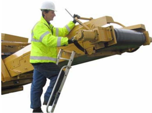
19: Raise main conveyor spray bar to working position.
