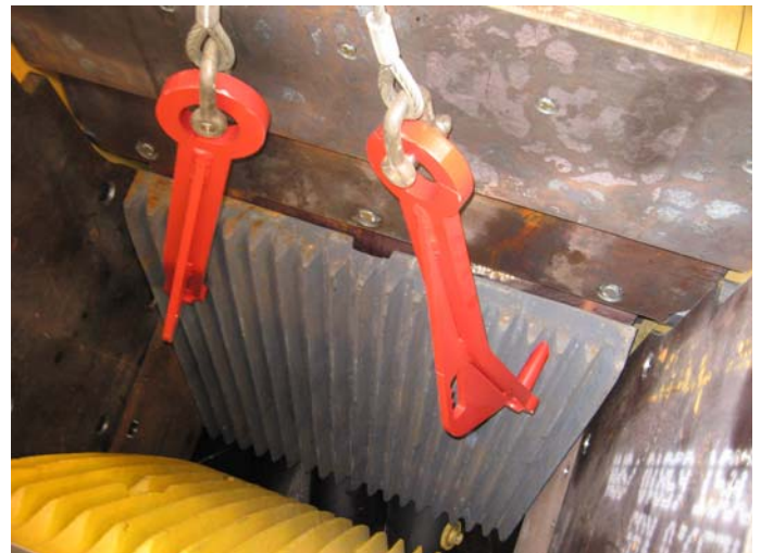
6: The jaw plate recesses will audibly drop onto the location point.
