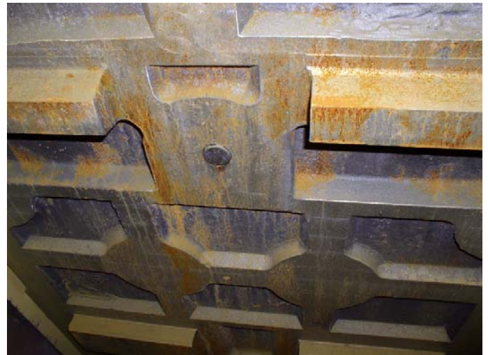
8: Ram pin fully back. Clean mounting plate.
