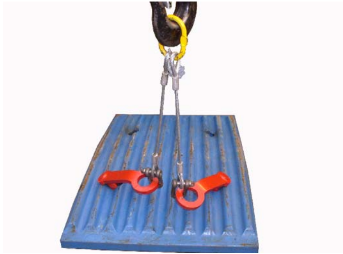
1: Place lifting tools in jaw plate. Before lifting the plate ensure the back face and pockets are clean of debris.
