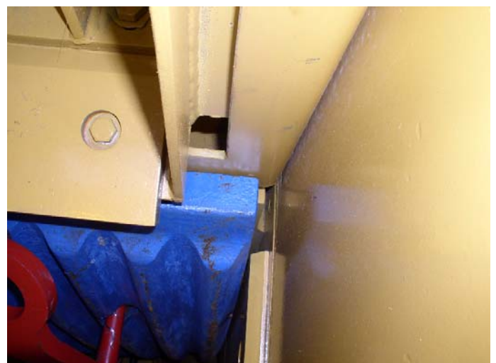
14: Visually position the fixed jaw plate against the sealing plate. (C-10 Only.)
