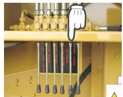
6: Activate levers to raise rear jacking legs.
