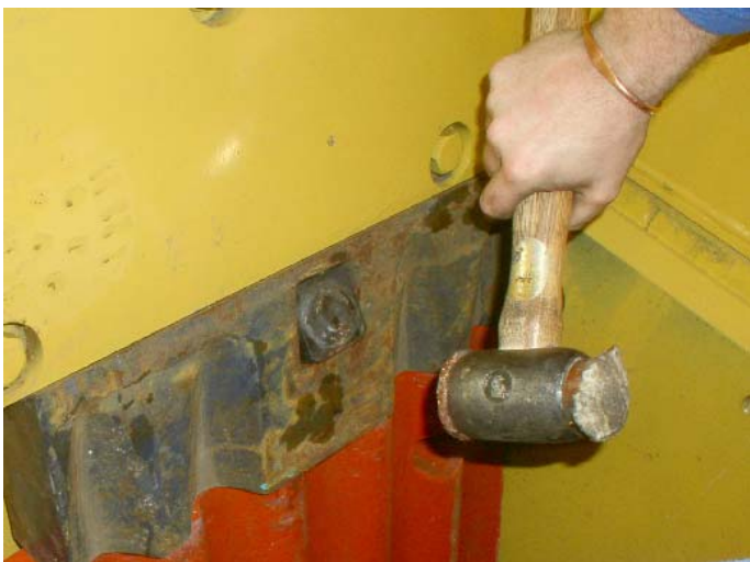
13: Knock home wedge bolt. Repeat steps 10 to 12 for the opposite wedge.
