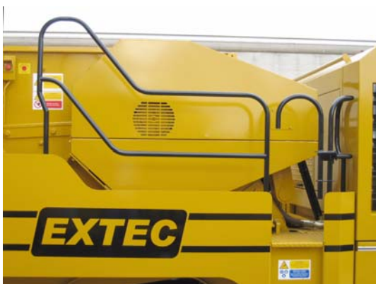
1: Look through slotted area on guard at alignment arrow on shaft end plate.
