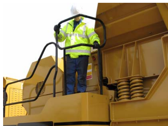
22: Lift rail into position and lock with pin.
