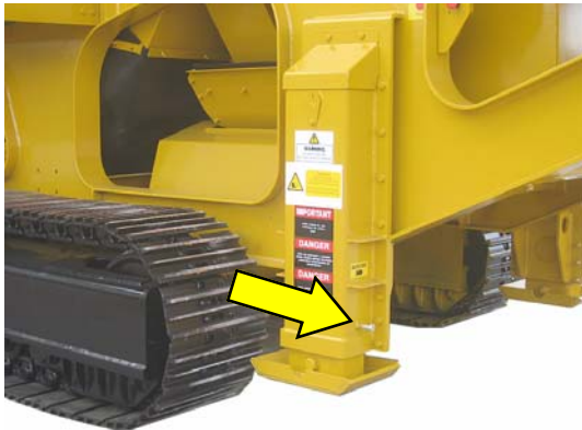
1: Remove jacking leg retention screws.
