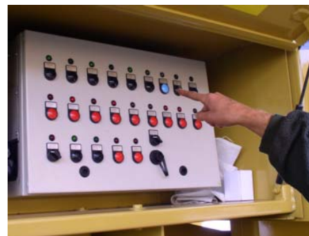
8: Press button TRACKS ON.
