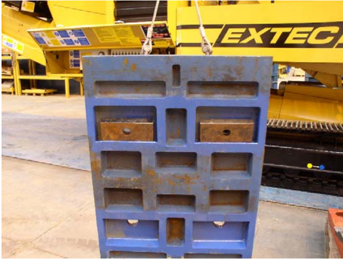
5: Wedges in place and lined up.
