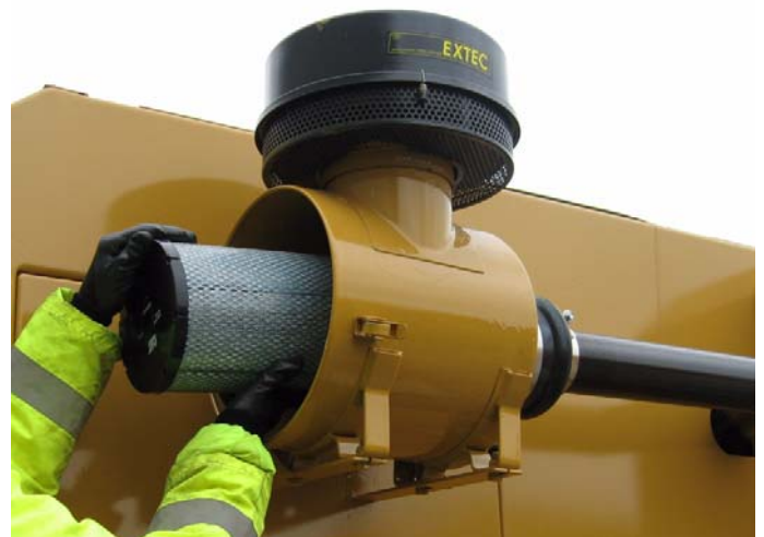
4: Only remove and replace secondary air cleaner after three services. (EN1004)
