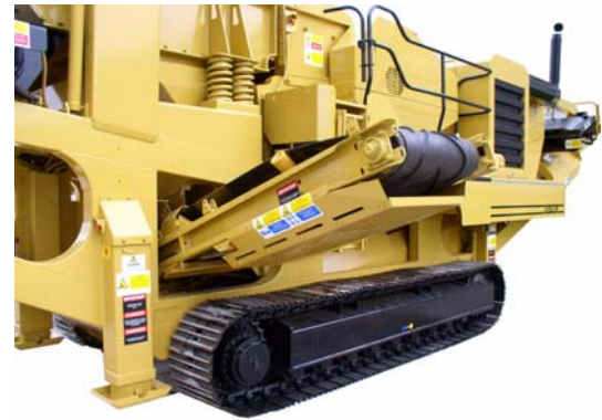
16: Side conveyor in working position
