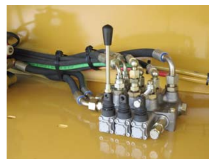
15: Remove valve handle and lock back into position shown above.
