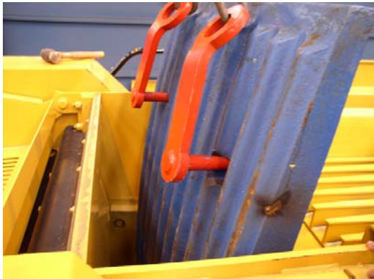
3: Remove jaw plate using lifting hook & ropes provided with machine and suitable lifting equipment.
