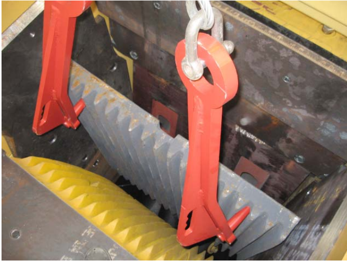
11: Lower fixed jaw plate slowly into the crusher box. Stand well clear off the jaw plate.
