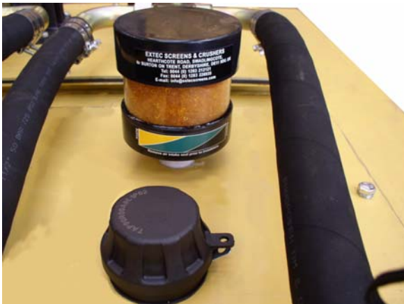
1: Raise cover plate and examine service indicator.
