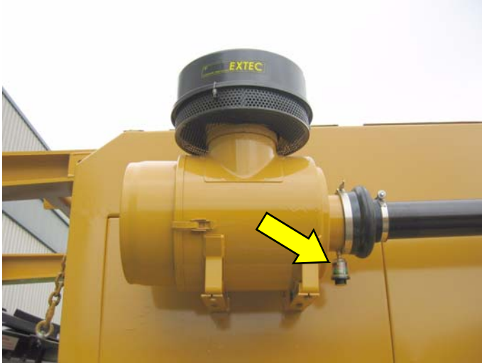
1: Check the service indicator daily. (EN1008)
