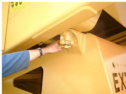
5: Unlock bogie from machine (4 positions).
