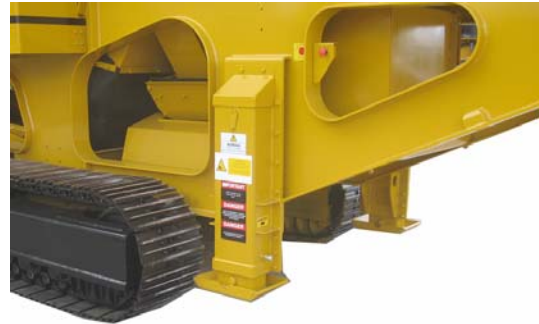
7: Lower rear jacking legs to raise machine clear of the bogie locking mechanism.
