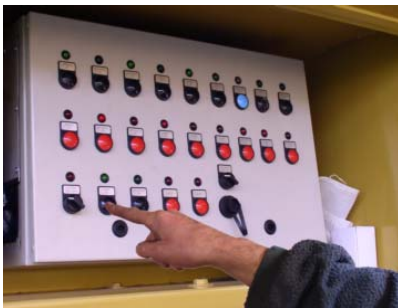
1: Press button CLAMP ON.
