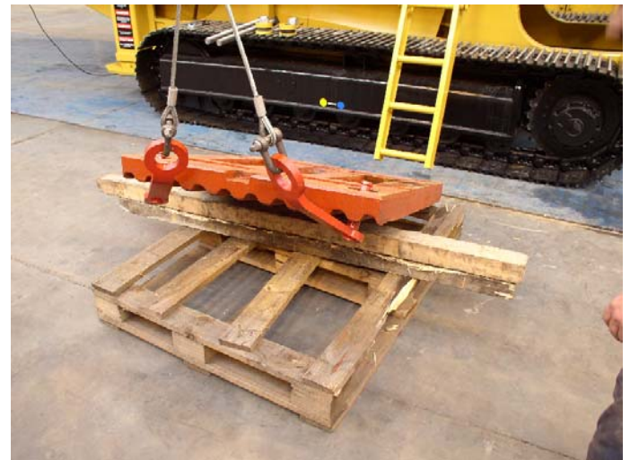
2: Lift swing jaw plate as shown. Clean face and pockets of the jaw plate first before lifting.
