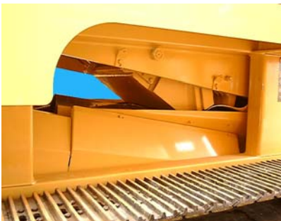
4: Main conveyor in raised position
