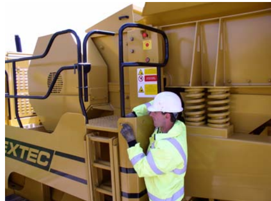
22: Lift rail into position and lock with pin.
