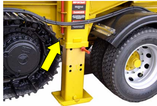
1: Remove jacking leg retention screws.
