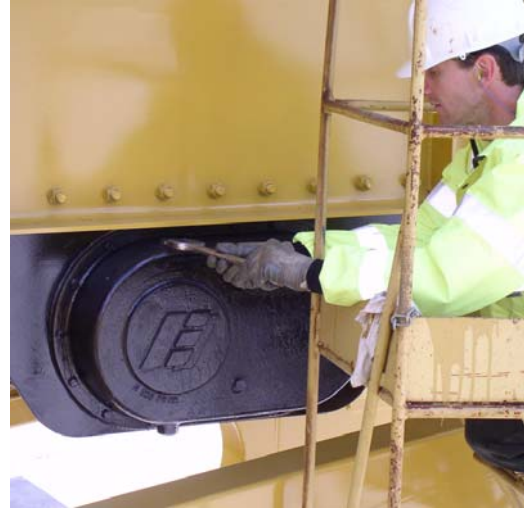
2: Remove oil filler plug.
