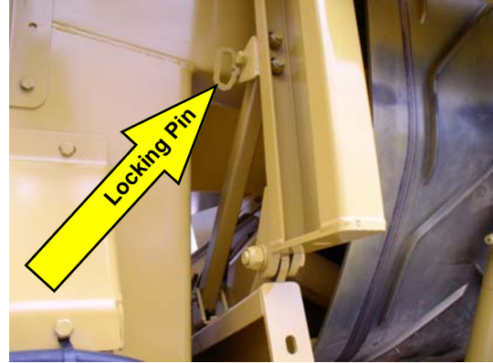
14: Remove side conveyor locking pin.
