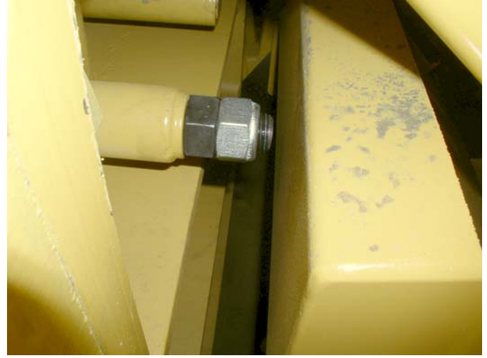
18: Tighten plain nut and torque. Lock after with Nyloc nut.
