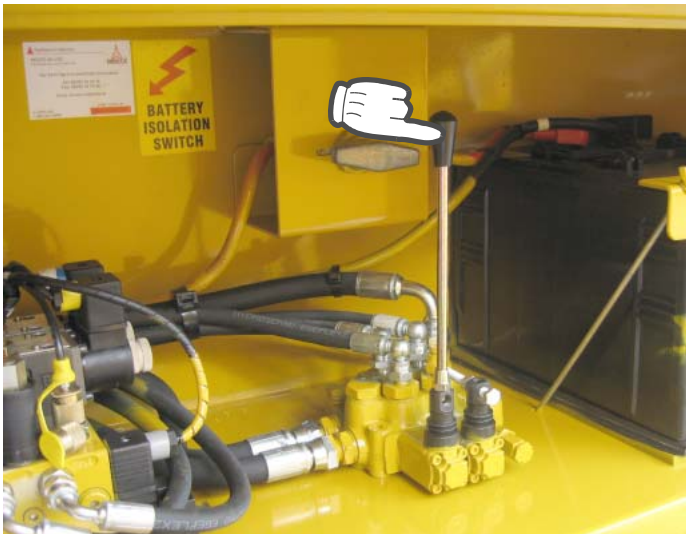
7: Pull wear plate release lever to move wedge rams back into position.
