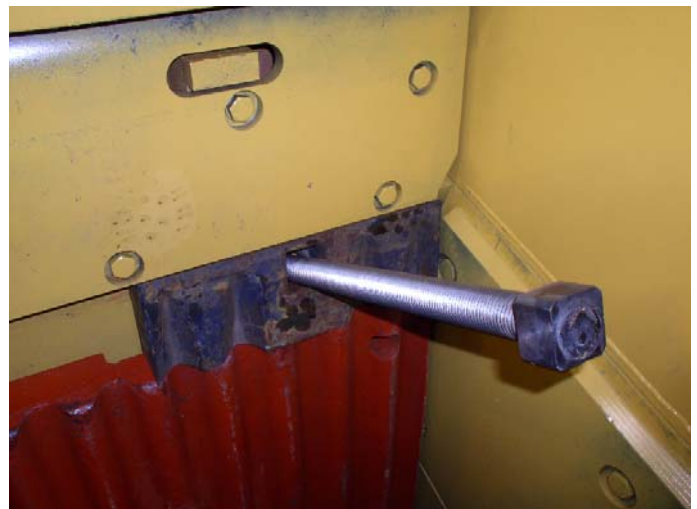
12: Carefully slide the wedge into position. Remove bar and slide wedge bolt into place.
