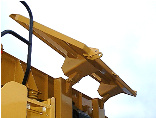
7: Hopper side door being raised.
