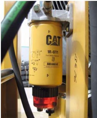
5: Bleed diesel water trap. (EN1002)
