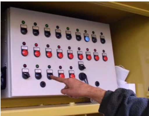
3: Press button JAW ADJUSTMENT ON.
