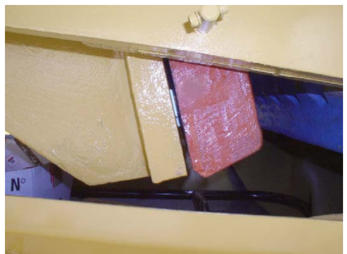
8: The photo show a gap at the bottom which is incorrect. Plate must be flush with jaw face.
