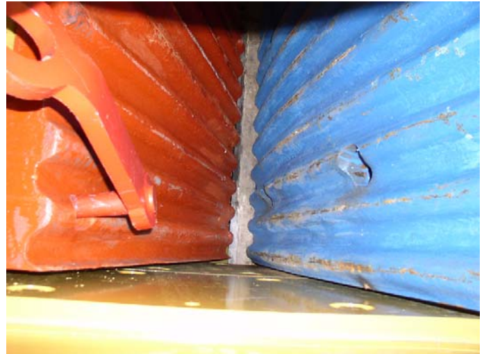
10: Adjust plate position using lifting equipment.
