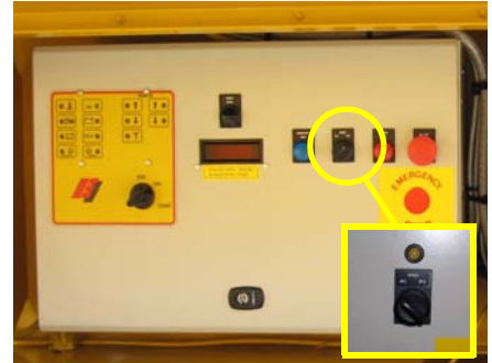
6: Restart the machine and leave speed switch at position No.1. Do Not Operate the Jaw Lock.
