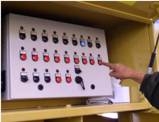
3: Press button MAIN CONVEYOR LOWER.
