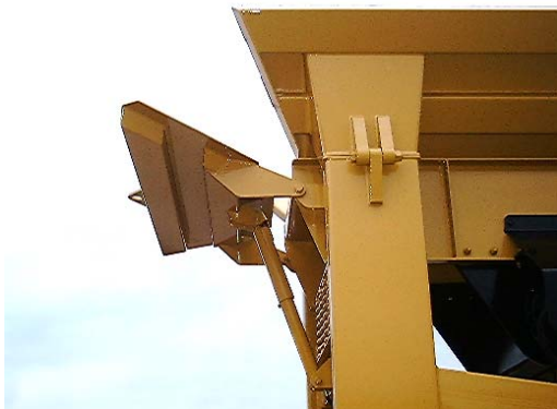
14: Hopper back door being raised.
