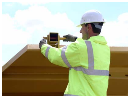
12: Fit hopper cross-tie box and secure with pins and R-clip.
