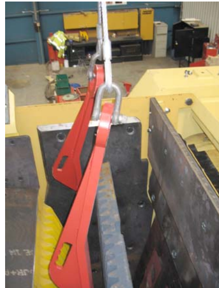
6: Remove jaw plates using lifting hook & ropes provided with machine and suitable lifting equipment.
