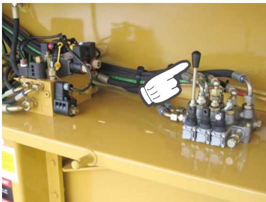
17: Raise main conveyor.
