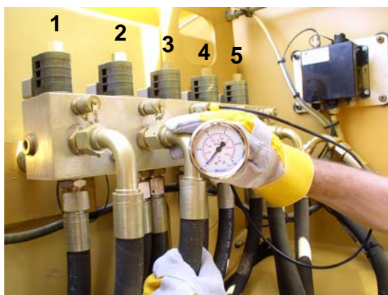
Figure 6-1: Test points are on manifold block on side of valve plate.
