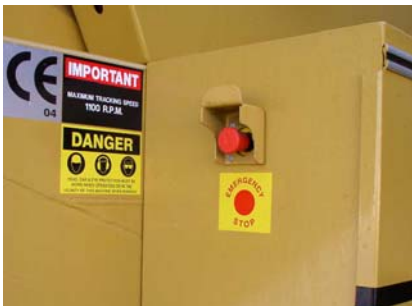
5: Emergency stop on control box
