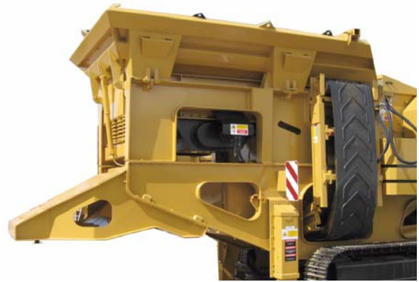
10: Hopper sides fully raised.
