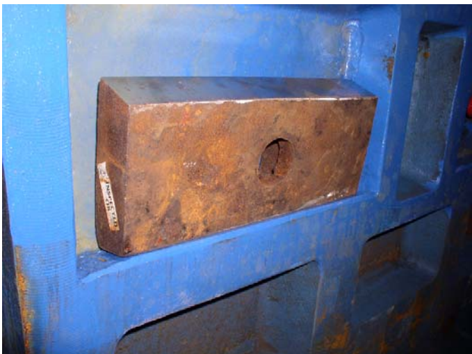
4: Place wedge in recess. The wedge should not rest on the lifting tool. See above photos for approximate position.
