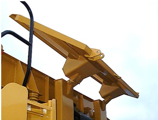
12: Hopper side door being raised.
