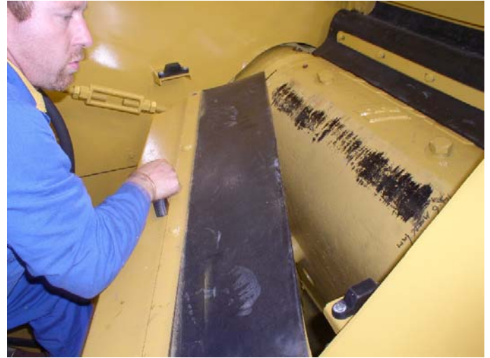
16: Refit toggle cover plate and guard.
