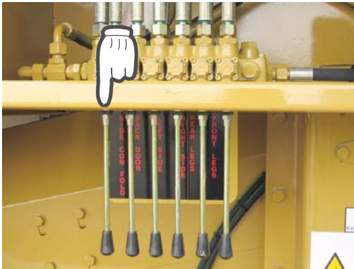
15: Activate lever marked SIDE CON FOLD to lower side conveyor.
