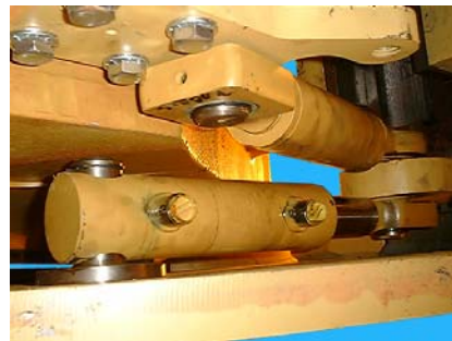
11: Examine toggle clamping and lift ram bearings for cracks due to toggle replacement. Replace if necessary.
