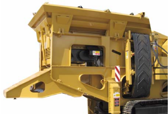
15: Hopper sides fully raised.
