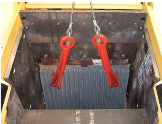
3: Remove wedge bolts and wedges from swing jaw stock only.
