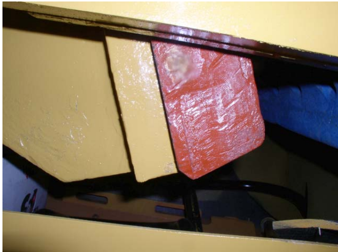
9: The photo show no gap at the bottom which is correct. The plate is flush with jaw face.
