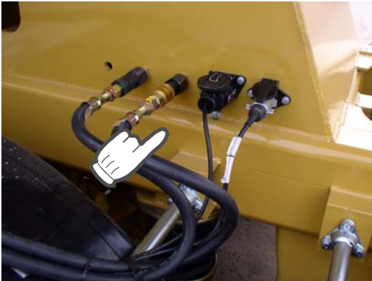
8: Remove bogie air brakes & lighting connections then tow away from machine.
