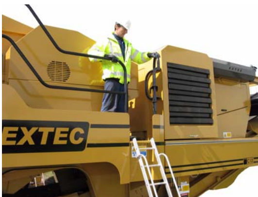
23: Lift up rotating gate section, rotate & lower into position. Repeat the procedure on other side of machine.
