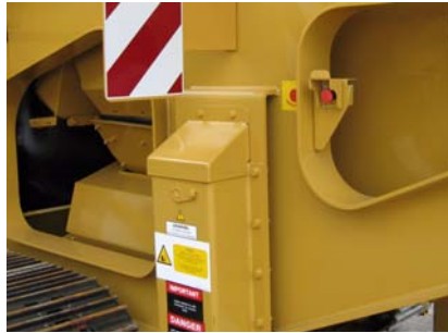
2: Emergency stop on L/H & R/H jacking legs
