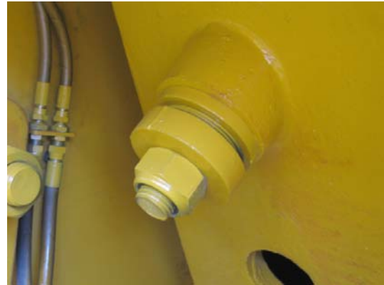
2: Loosen and remove the wedge bolts.
