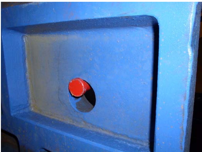
2: Ensure the lifting tool catches in the hole. Lift jaw plate with suitable lifting equipment.
