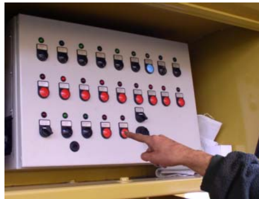
4: Press button JAW IN to close up jaw.
