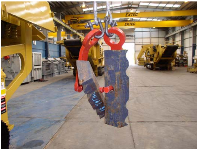
1: Lift wedges onto machine.
