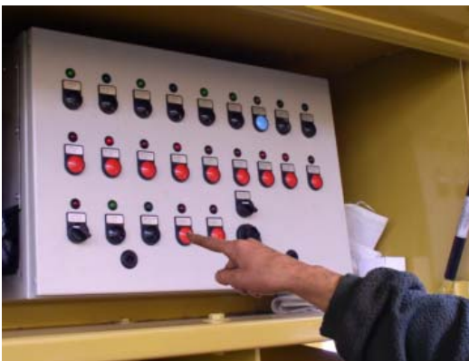
5: Press button JAW OUT to open up jaw.
