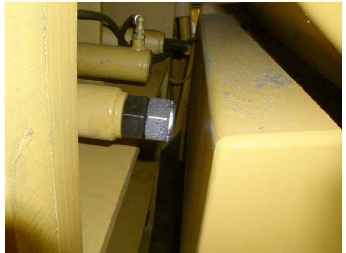
16: Screw on both nuts before tightening.
