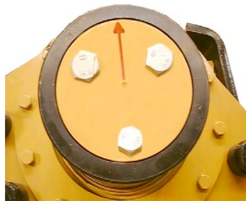
2: Alignment arrow points vertically up at minimum jaw opening.
