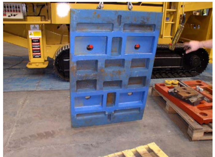
3: Ensure back of the plate is clean and smooth. Clean out any accumulated debris in the recesses.
