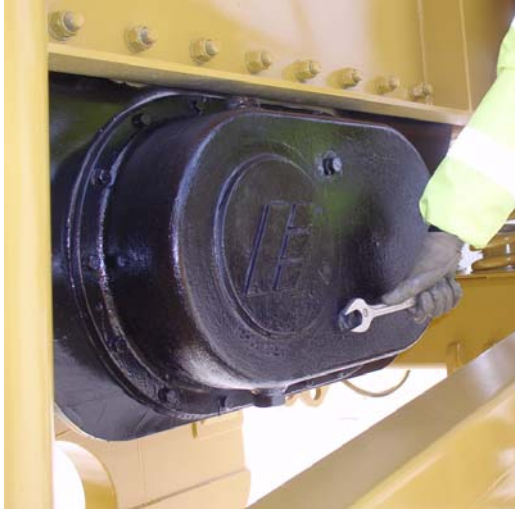
1: Remove oil level plug.
