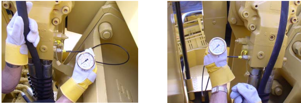
Figure 6-2: Checking Control Block Pressure
