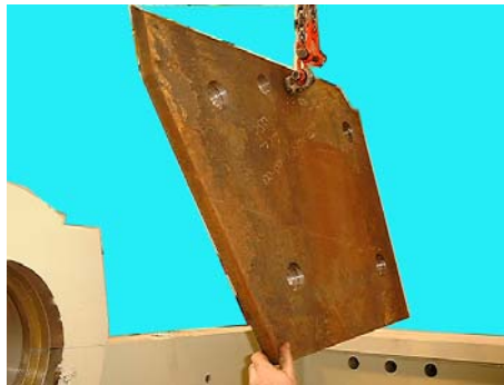
1: Changing Liner Plates
