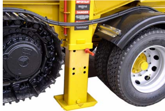
7: Lower rear jacking legs to raise machine clear of the bogie locking mechanism.
