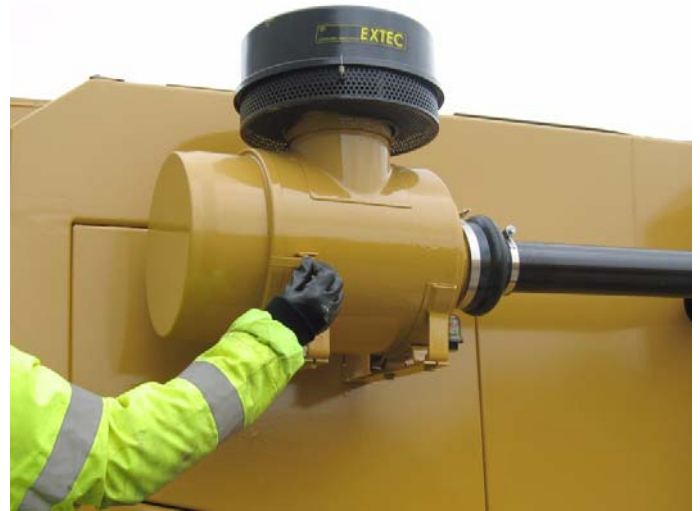
2: Unclip the cover and remove.
