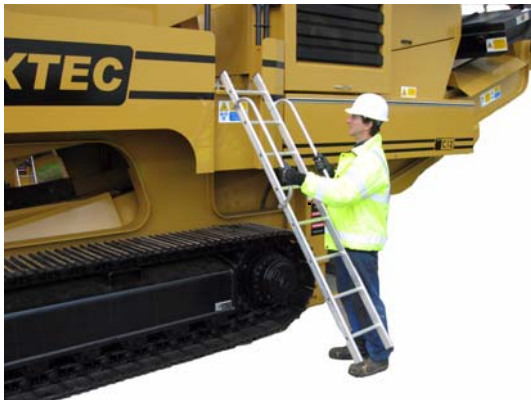
21: Unfold ladder, ensuring its locked into position.
