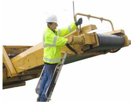
20: Fix main conveyor spray bar in working position and secure.
