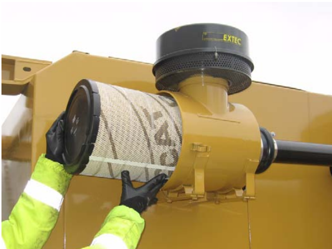
3: Remove and clean the primary air cleaner. The primary air cleaner can be used up to six times if properly maintained. Replace at least once a year. (EN1003)
