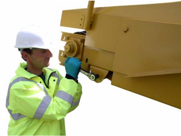
Figure 5-1: Adjusting Belt Scraper
