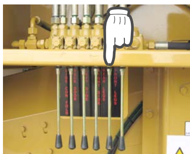
25: Lower rear jack legs by operating levers.
