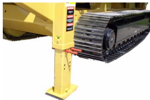
2: Ensure that locking pins and R-clips are fitted BEFORE cleaning below the machine.
