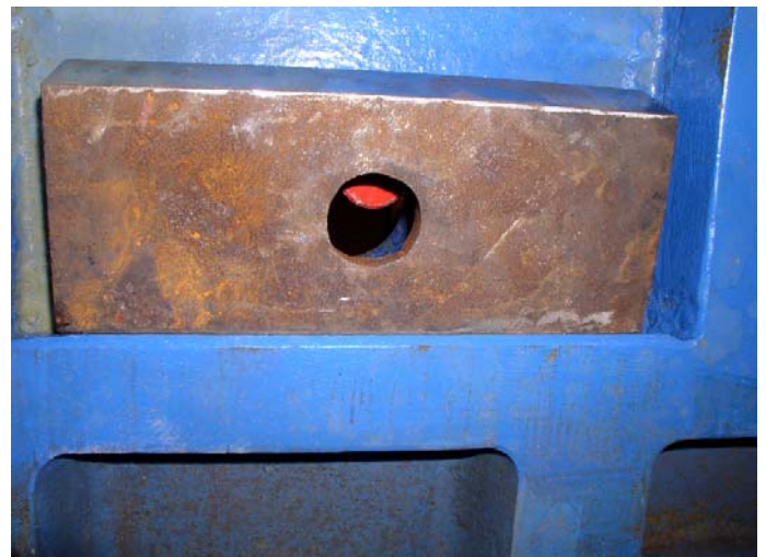
4: Place wedge in recess. The wedge should not rest on the lifting tool. See above photos for approximate position.
