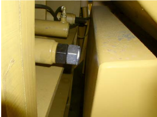
1: Remove locking nuts to remove fixed jaw plate.
