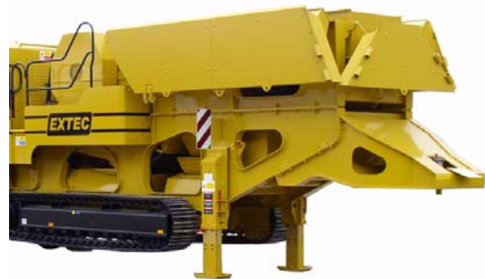
3: Lower front jacking legs to raise fifth wheel neck by approximately 100 mm.
