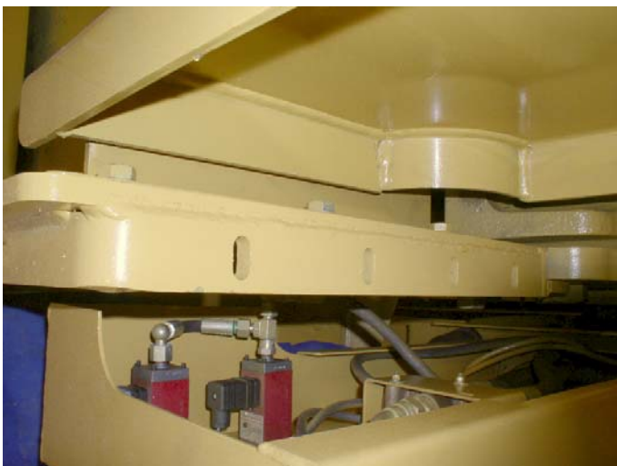
9: Loosen bolts on sealing plate. (C-10 Only.)
