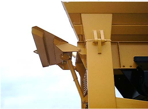
9: Hopper back door being raised.
