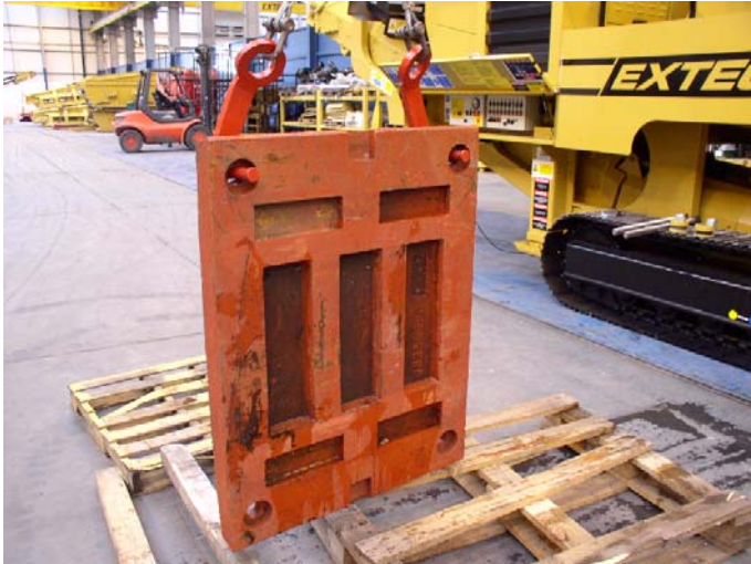
3: Position of hooks after jaw plate lifted
