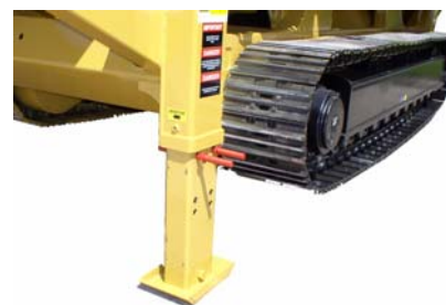
27: Fit pins & R-clips to jack legs (8 off).
