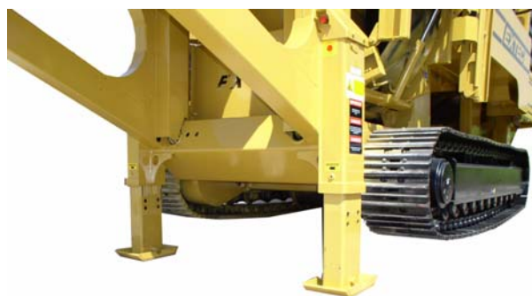
1: Using jacking legs, lift the machine off ground.
