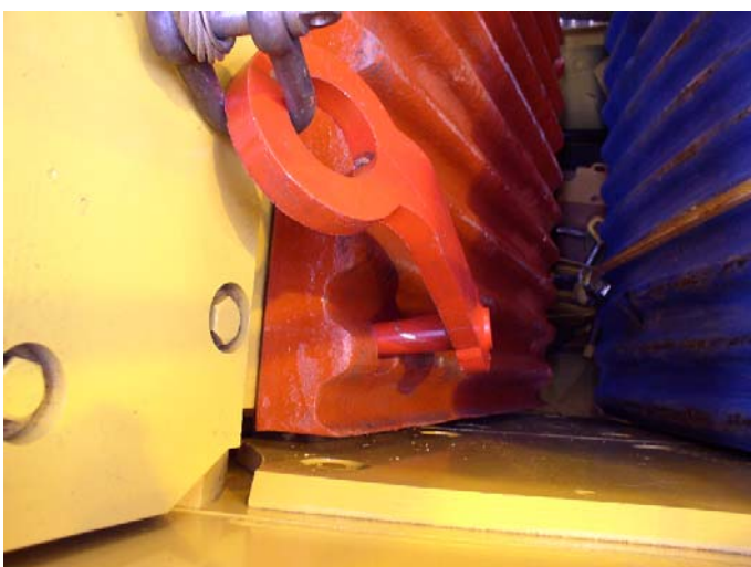
7: Ensure a even gap on both side. The jaw plate must be flush with the mounting face.
