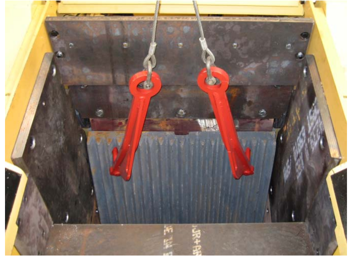
12: Leave a 10 to 15 mm gap on either side of the jaw plate.
