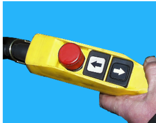
2: Remote pendant for opening jaw
