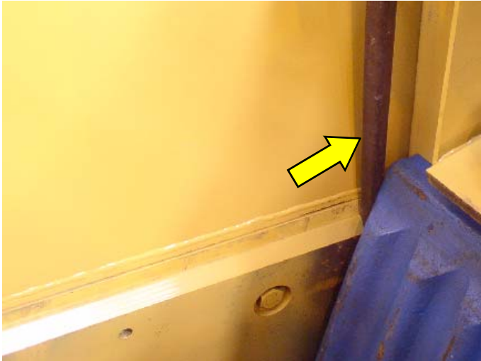
17: Using a suitable pry bar check plate for central position.
