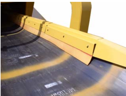
1: Sealing rubber in correct position & condition
