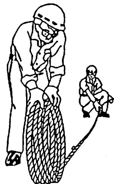
Unreeing method of wire rope
