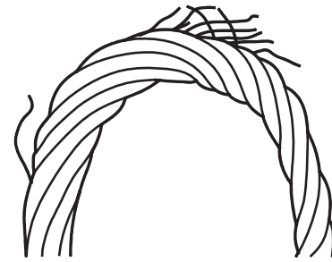
Band rope sharply to expose breakage
