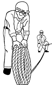
Unreeving method of wire rope
