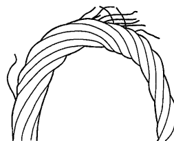
Bend rope sharply to expose breakage.
