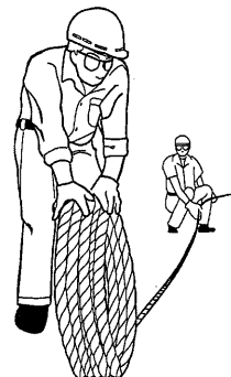
Unreeving method of wire rope
