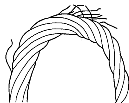
Bend rope sharply to expose breakage.
