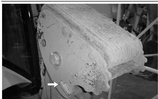
Illustration 112 g01033442 The grousers are facing downward.
