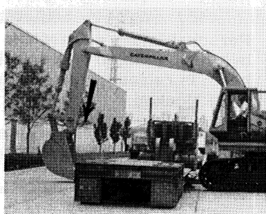
2. Apply down pressure on boom. Raise the front of track clear of trailer bed.
