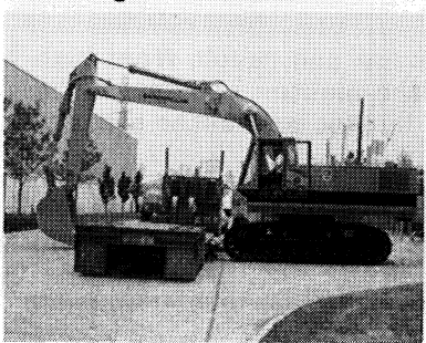
1. Position machine so front is facing side of trailer. Position boom over opposite side of trailer.
