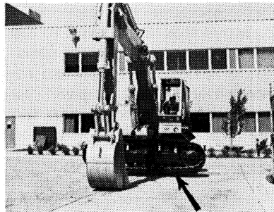
2. Apply down pressure on boom to raise track clear of ground.
