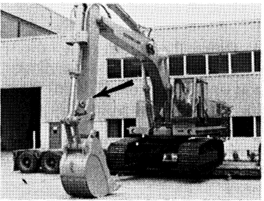
5. Move stick out and move rest of machine onto trailer.
