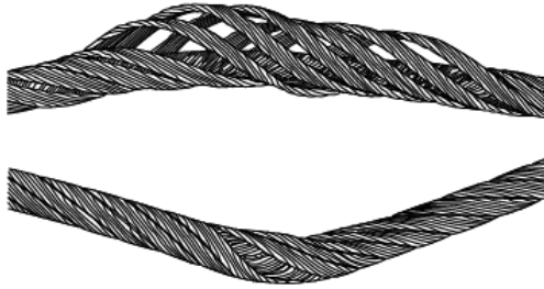
Figure 154: Example of damaged wire rope
