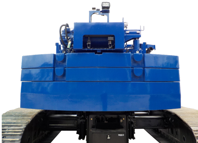
Figure 77: Upper counterweight installed
