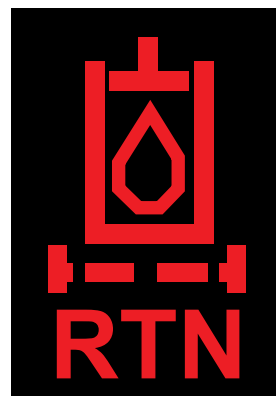
Return filter clogged
