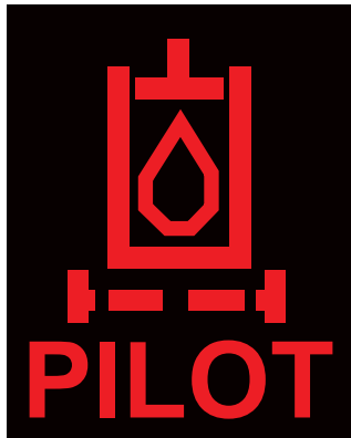
Pilot filter clogged
