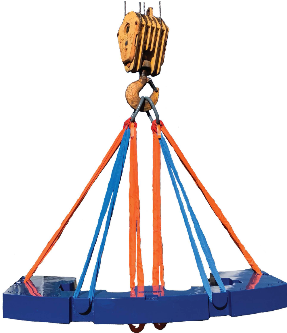
Figure 74: Lifting upper counterweight top section
