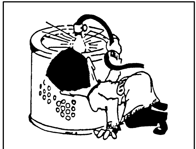
Figure 2-12 Inspecting the Air Cleaner Element
