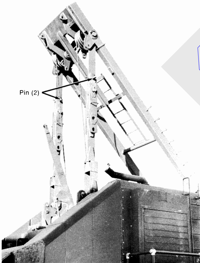
Figure 1. Gantry shown in Lift, Clam, Drag Working Position
