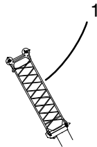
K 18 ft (5.5m) Fly Extension With Lifting Sheaves
