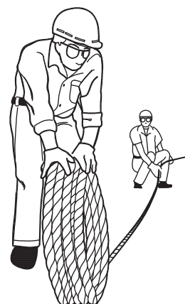
Unreeving method of wire rope
